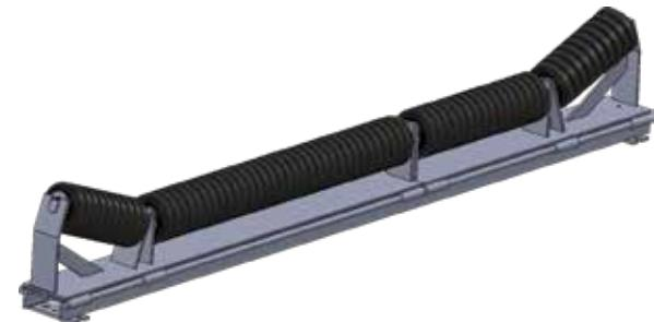
**Sliding Station:** To be used in areas where assembly and maintenance is difficult, the sliding structure with rollers on a fixed body facilitates maintenance and assembly. If there is a load on the belt, we can additionally take the load of the belt and facilitate the aquaplaning movement with the jack systems. Skid stations can be manufactured in special sizes for each conveyor.
