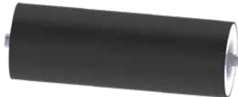
**Rubber Coated (Vulcanized) Roller:** This roller absorbs the pressure and shock created by falling materials in large material conveyor systems with heavy-duty conveyor belts. It is formed from a steel roller with hot vulcanized coating on roller.
